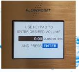
3. Access combo correct, enter in the desired volume and hit ENTER.
