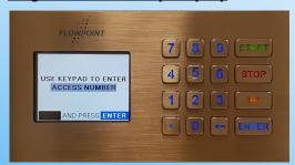
1. Using the Keypad, type in the Access code and then ENTER.
